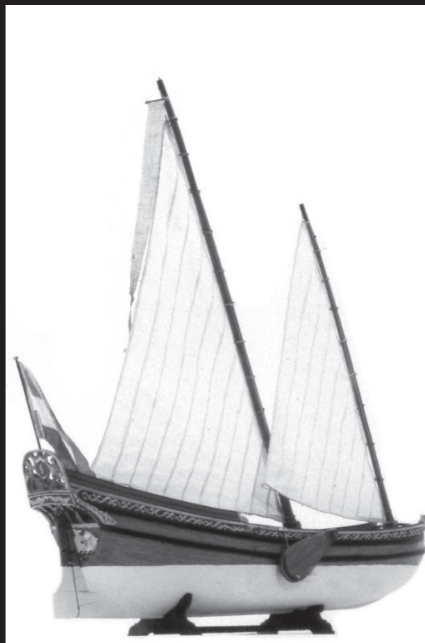
Model of a 42-feet pleasure yacht by Ab Hoving built after a contract in Nicolaes Witsen: Aeloude en Hedendaegse Scheepsbouw en Bestier , 1671, Amsterdam. p. 175. The rig consists of two loose footed triangular sails.
